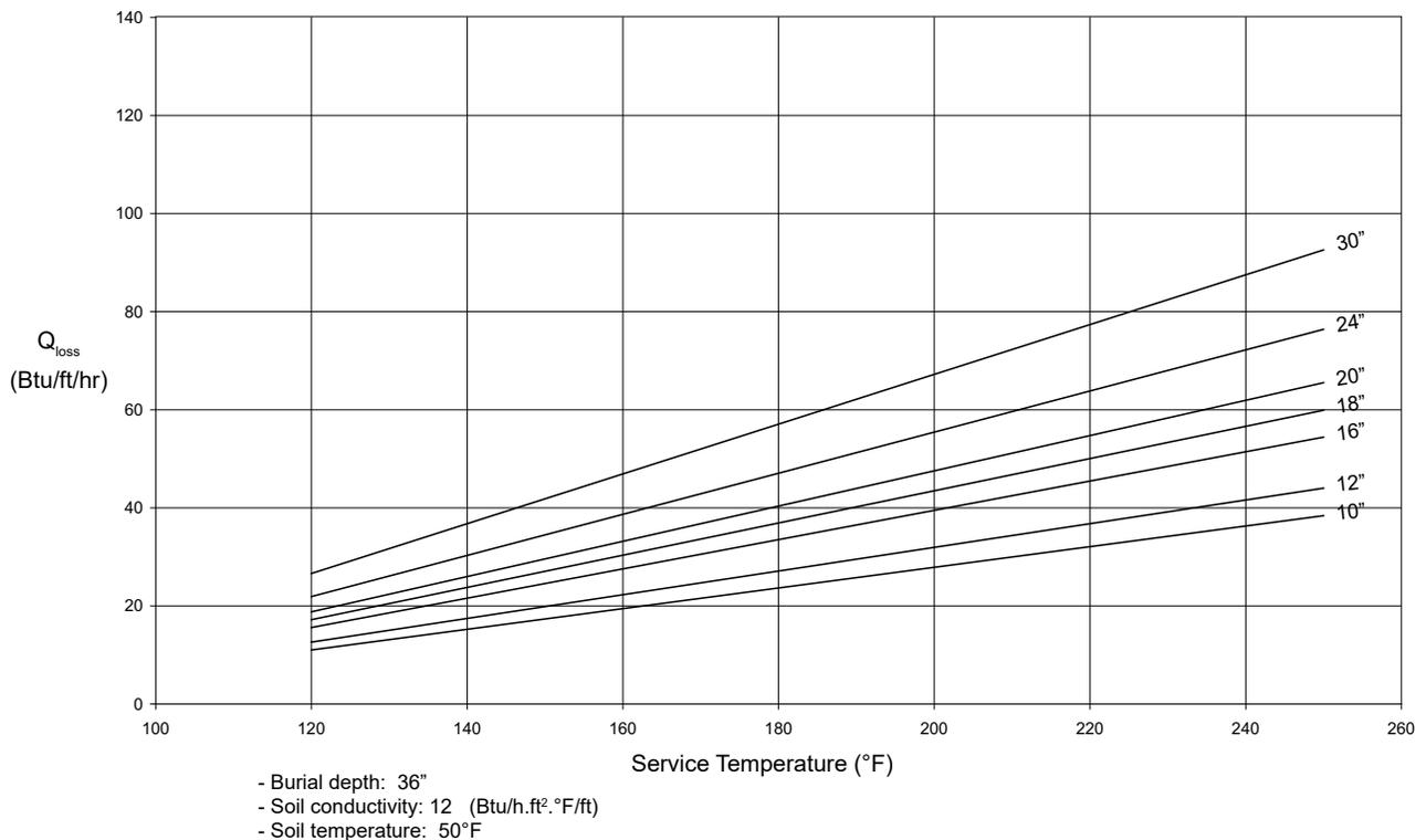
\* Values are calculated using 3E Plus in accordance with ASTM C680 and are subject to the terms and limitations stated in the software. Actual heat loss may vary.
