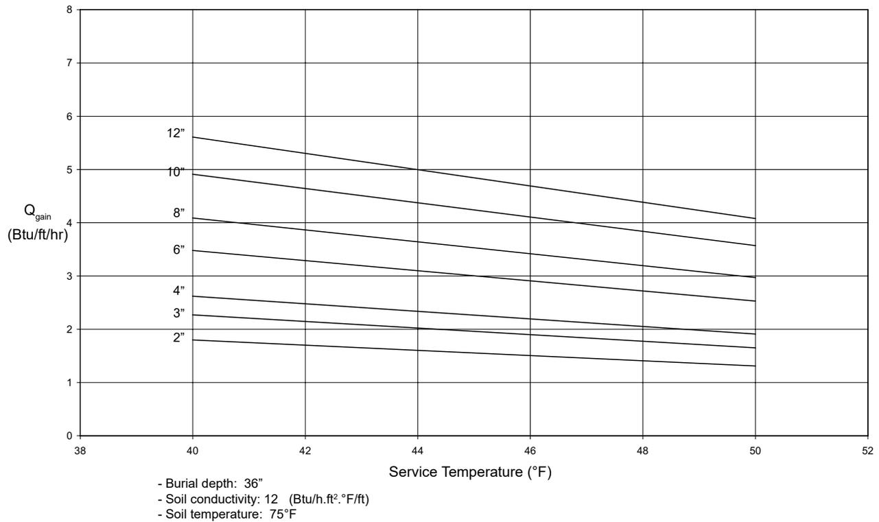
\* Values are calculated using 3E Plus in accordance with ASTM C680 and are subject to the terms and limitations stated in the software. Actual heat gain may vary.
