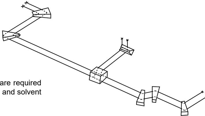
NOTE: Thrust blocks are required with solvent weld pipe and solvent weld fittings.
