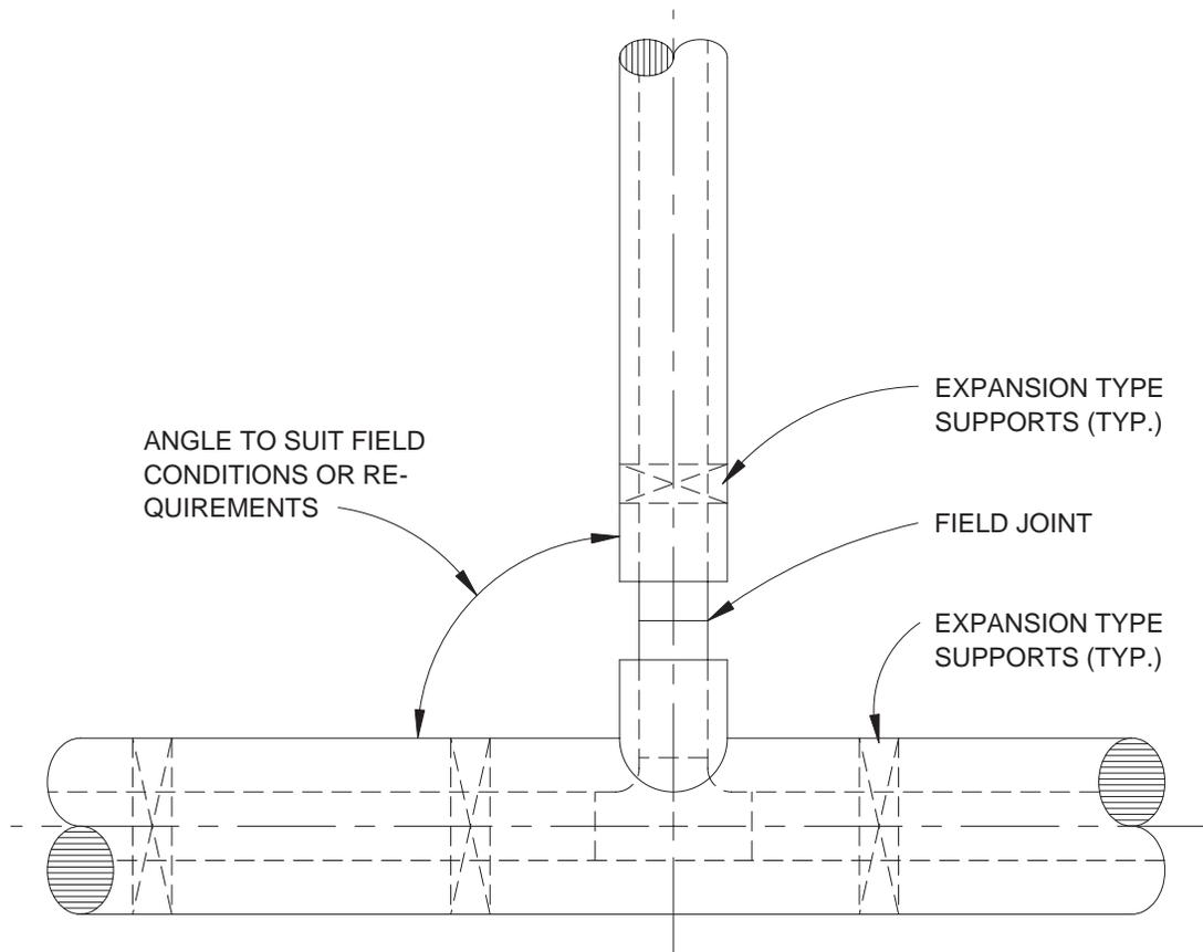
NOTE: LIMITED EXPANSION TEE TO BE USED ONLY IN UNUSUAL OR ISOLATED APPLICATIONS SUCH AS WHERE MANHOLES OR OTHER CONNECTION DEVICES ARE PROHIBITIVE. REF. SK-3 OR SK-5 TYPE B EXPANSION SUPPORTS.
