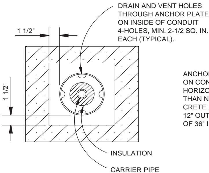
ANCHOR PLATES ARE 1/2" STEEL CENTERED ON CONDUIT WITH DIMENSIONS 1 1/2" LARGER HORIZONTALLY AND 1 1/2" LARGER VERTICALLY THAN NOMINAL CONDUIT DIAMETER. CONCRETE ANCHOR BLOCK EXTENDS MINIMUM OF 12" OUTSIDE ANCHOR PLATE AND IS MINIMUM OF 36" IN LENGTH.
