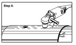
Apply firm downward pressure on the plug, then spin the plug at full speed until outside of drill bit touches HDPE jacket (approx. 13 seconds). Stop spinning the plug, but continue applying downward pressure for 20 seconds.
