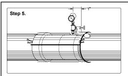
Push the Pressure Gauge and Valve Test Device into the hole. Using hand pump or other air supply obtain 5 psi pressure. Disconnect air supply and soap joint for "pin hole" leaks. Hold air pressure for 5 minutes. (Note: In rare cases air will escape down the interface between the foam and the jacket. This can be confirmed by soaping the end of the jacket interface).
