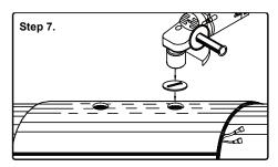
Clean any excess foam off the HDPE jacket. Using a chisel or other device, remove the foam from each hole to below the lip of the HDPE. Rough up surface using 80-grit sandpaper for proper fusion. Install drill bit provided by Thermacor into 5/8" side grinder. Fit the raised tongue of the white plug into the groove in the drill bit. Center the raised circle on the plug into the hole in the HDPE jacket.
