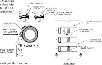
Place one hand on the rubber band below the buckle as shown and pull the loose end of the rubber band to apply pressure to the seam of the PTJC sleeve. Continue pulling until a 1"- 2" gap appears between the Rubber Band Overlap and the Joint Overlap (B).
