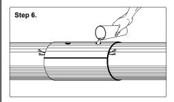
Remove test apparatus. Drill a second 1" hole 10" from the 9" mark at 12 O' Clock. Mix required foam per Foam Kit Instructions and pour into 1" hole. Allow foam and gas (Air) to escape through holes, cover the holes with duct tape when the foam comes out of the holes. See Foam Kit Instructions for quantities, etc.
