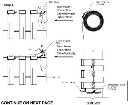
Connect 110V single phase welding machine to a <u>PEDICATED POWER SOURCE</u>. Attach power cables extending from a 110V single phase welding machine to the Electro-Fusion wire. (Note: It does not matter which color power cable is connected to the Electro-Fusion wire). 2 white on one side, 2 black on the other side.
